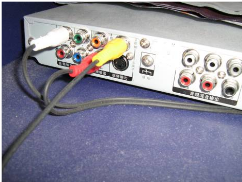
Figure 2: Incorrect connection of devices
