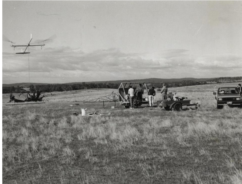
Figure 2: Gyromill Mk2 during low-level flight at the University of Sydney's Mt. Pleasant farm
