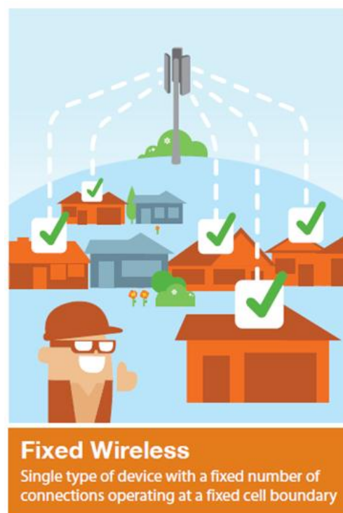
Figure 6: Fixed wireless distribution topology
