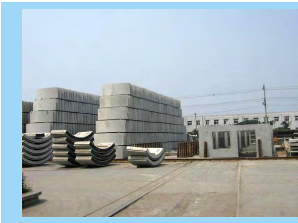
Figure 18 Prefabricated concrete structural products at case study factory yard
