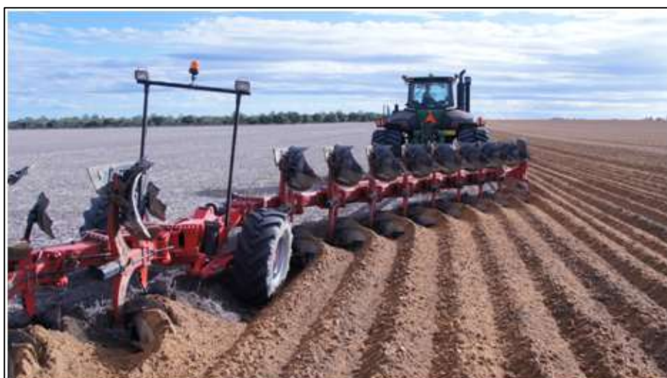
Fig. 6. Over-cultivation with implements, such as the disc plough, is a major cause of soil structure decline. Source: www.agric.gov.au
