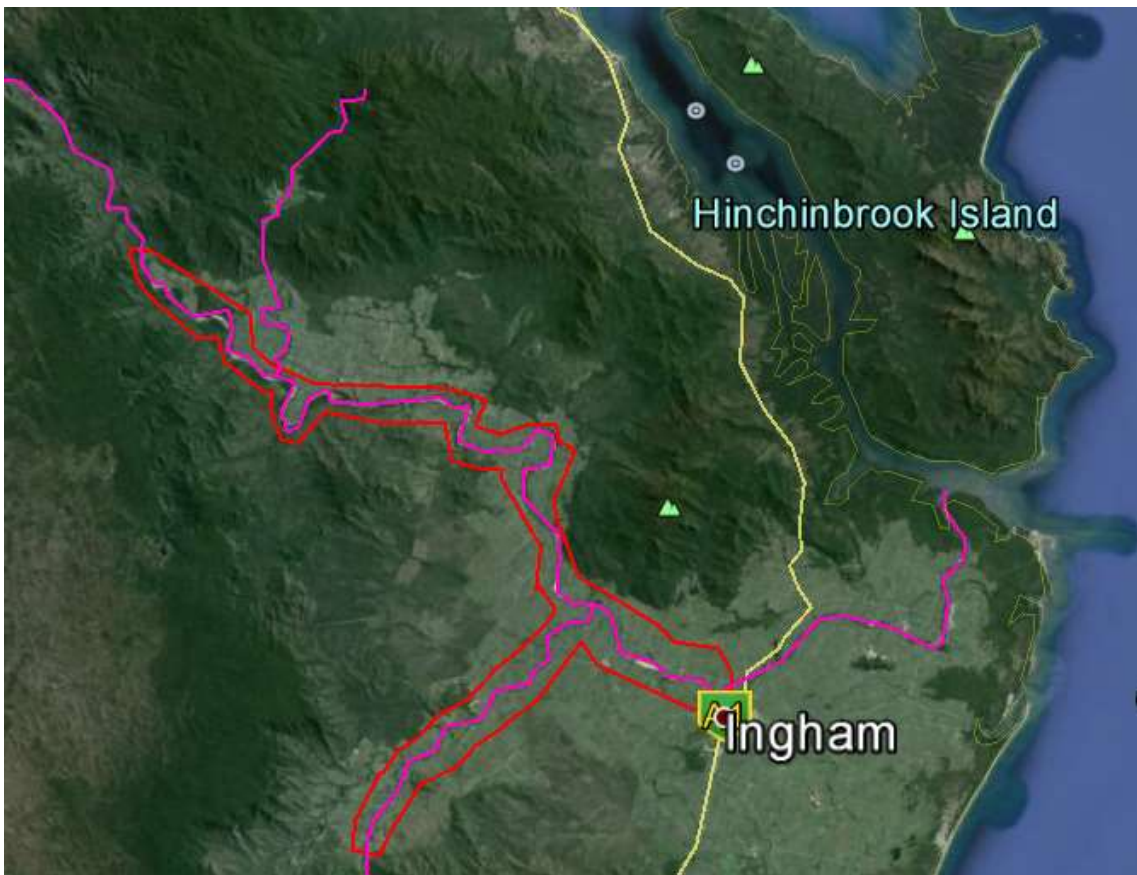
Figure 78. The area of streambanks to be remediated in the Herbert River - 5% (top), 10 % (bottom). Existing vegetation coverage in the proposed restoration zone was estimated to be 40% and 20% respectively.
