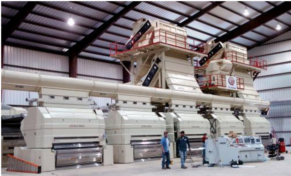
Figure 2: Commercial cotton gin operating in the USA. Source: Lubbock Avalanche-Journal, Flickr.
