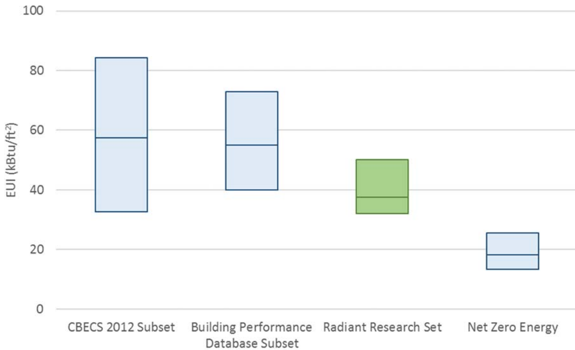
Figure 5: Box plot bounding 25 th and 75 th percentile EUI of the research set and various benchmarks
