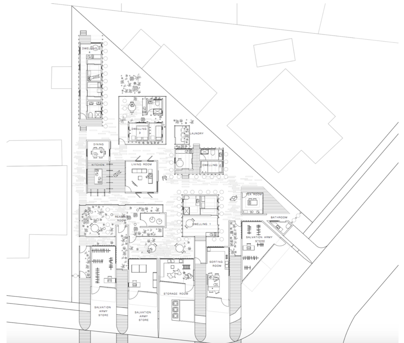
Figure 3: Plan of Patane’s Chimera scheme. Illustrated here in mixed use mode, the garages along the street edge are converted into a Salvation Army Opportunity Shop, providing income and employment opportunities for occupants whilst simultaneously screening the refuge behind. Living quarters are broken up into functions with un-habitable spaces occupying small sheds around habitable granny flats. Not to scale.
