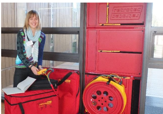
Airtightness is measured using blower door testing.
