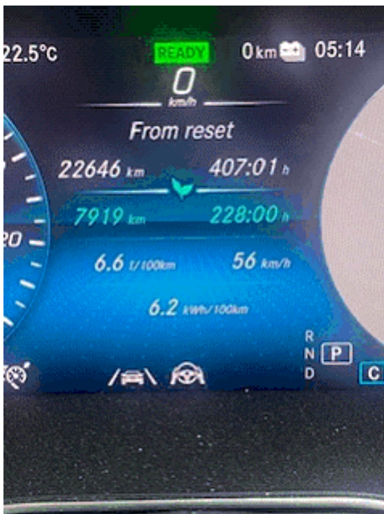
Figure 2: Odometer with separate readings for petrol and electric kilometres travelled
