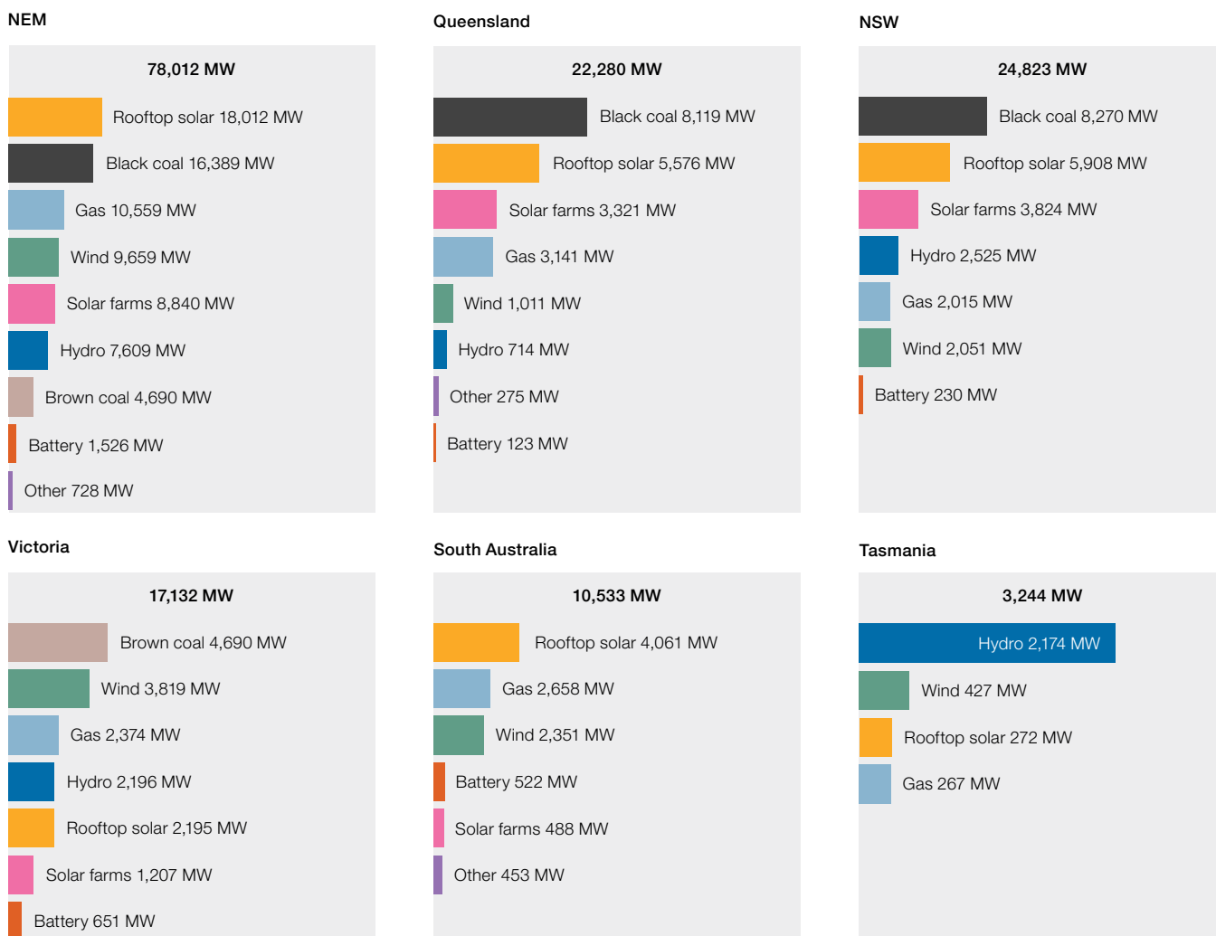
Figure 3.14 Generation capacity, by fuel source
