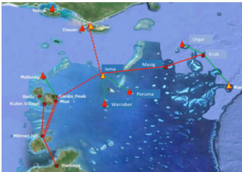
Figure 7: Map showing path of Telstra microwave repeater network (Source: https://tsirc.qld.gov.au/deputations/connected-islands )
