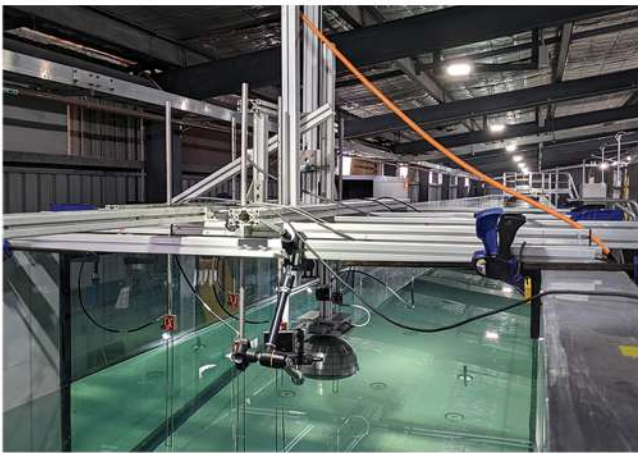
FIGURE 7.2 SETUP OF LABORATORY EXPERIMENT AT UWA'S COASTAL AND OFFSHORE RESEARCH LABORATORY TO INVESTIGATE NONLINEAR INTERACTIONS BETWEEN WAVES AND A WAVE ENERGY CONVERTER
