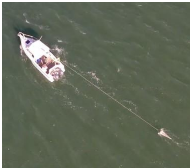
Figure 6 Manta net being towed by 6.4-metre vessel. NSW EPA
