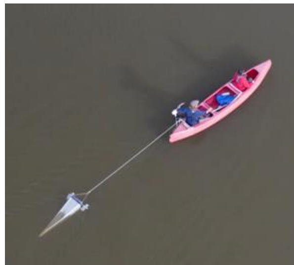
Figure 7 Manta net being towed by 4-metre canoe rigged with a motor on Parramatta River. NSW EPA
