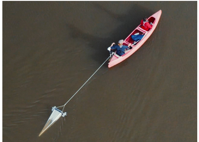
Manta net being towed by 4-metre canoe rigged with a motor on Parramatta River. Photo: NSW EPA
